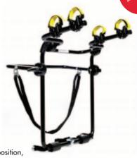
The rack once removed from the box, is to be set up in the above position, and placed over the spare wheel of the vehicle as pictured above. Ensure the spare tyre of the car fits completely into the rectangular bar of the rack. Wrap the retaining strap around the underside of the spare tyre and pull it tight, securing the rack to the tyre. A knot can be tied in both ends of the strap for additional security as pictured below.
