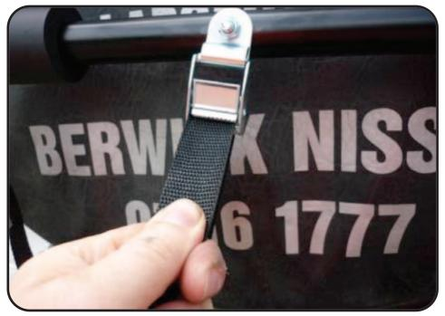
The remaining two straps can be used to secure the bikes to the rack once they are positioned in the cradles. Check the straps for wear and tear each time the rack is used. Ensure your vehicle's number plate is not obscured by the rack or the bicycles. If it is not clearly visible, ask your retailer about mounting your number plate to a rack mount with tail and brake light. (Available separately)
