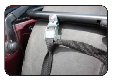
There are three straps along the bottom bar of the rack. The middle of these straps is used to secure the bottom of the rack to a suitable anchor point on the vehicle. A knot can be tied in the excess strap as above for additional security.
